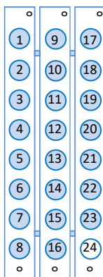
Figure 3. Positions of the 23 qPCR master mixes in each block of 3 x 8 tubes. Tube number 24 is empty and can be used for orientation of the 24 tube block. The hole in the upper right corner of each 8-tube strip (depicted as °) marks the beginning of the strip and the centered hole marks the end of the strip. The tube numbering refers to the tube numbering in the Interpretation table.
